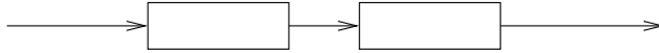
Figure 12.2: System components in series have the same average flow rate through each component, assuming that the system is running in a steady state – otherwise the pressure in the system would build up somewhere in one component, which would eventually cause a failure (like a burst pipe).
